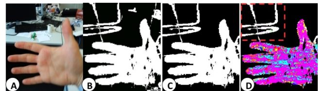
Figure 4: Segmentation by classification. A) Input frame. B) Foreground mask after color thresholding. C) Salt'n'pepper noise is cleaned up by connected component analysis; larger connected non-hand regions remain. D) Result after classification. Colored pixels indicate class label, white pixels indicate noise (red box).
