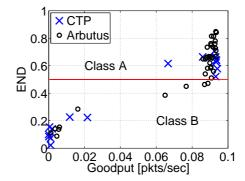
Fig. 3. With both CTP and Arbutus, the END metric generally correlates with the delivery rate, and the performance dichotomy shown in Figure 1 is confirmed. Low END values correspond to a less predictable performance.
