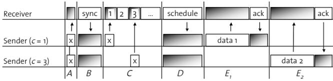
Fig. 3. Data SECTION with two senders transmitting a packet to the receiver. Cooperative transmission is used in segment A and single bit transmission in segments B and C to identify the senders.
