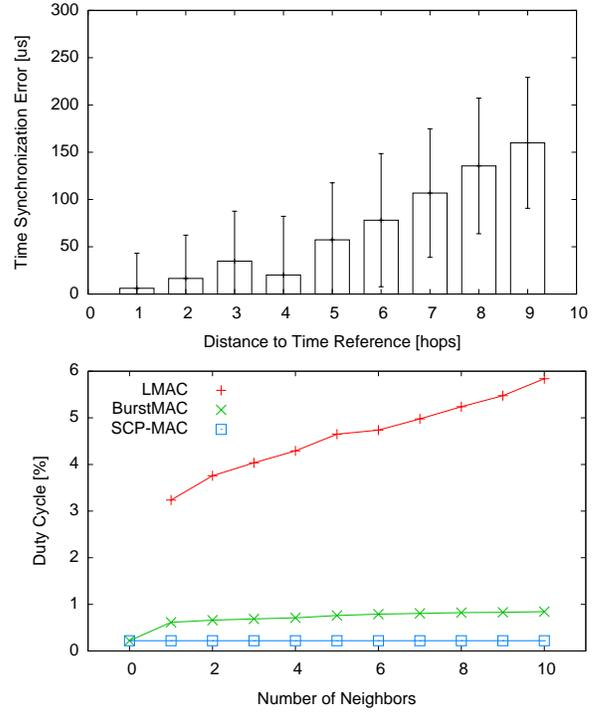
Fig. 5. Accuracy of BurstMAC time synchronization on a chain topology (top). Radio duty cycle in idle mode as a function of neighborhood size (bottom).
