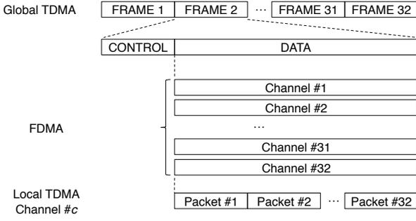
Fig. 1. BurstMAC protocol overview: Synchronous rounds consist of 32 frames (global TDMA). Each frame contains a CONTROL and a DATA section. Multiple radio channels are used for interference-free communication of collocated node clusters (FDMA). Communication within a node cluster is coordinated by local scheduling (local TDMA).
