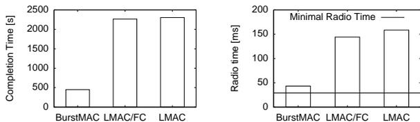
Fig. 8. Burst experiment: time to burst completion (left), average and minimal radio time per packet (right). LMAC/FC stands for LMAC with flow control.
