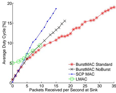
Fig. 6. Star topology with one sink and seven neighbor nodes: average duty cycle. Note that each protocol can only support constant traffic up to a certain packet rate.
