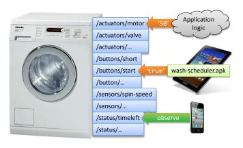
Figure 1. The thin server architecture to the extreme: A washing machine whose every button, actuator, and sensor is modeled as a resource. The application logic runs in the Cloud.
