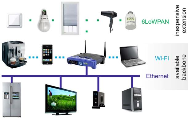
Figure 1. The architecture of IPv6-based HA
