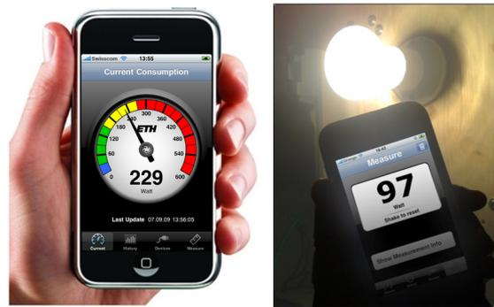
**Figure 5. Current consumption view of the mobile UI (left) and user determining the consumption of a light bulb (right)**
