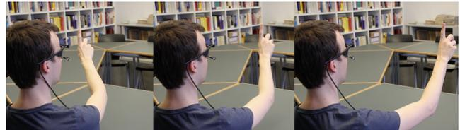
**Figure 1: Users can quickly and independently calibrate a head-mounted eye tracker by pointing with their fingertip at locations in the scene. No dedicated marker, display, or additional assistance is required, enabling a calibration technique suitable for mobile and pervasive eye tracking.**
