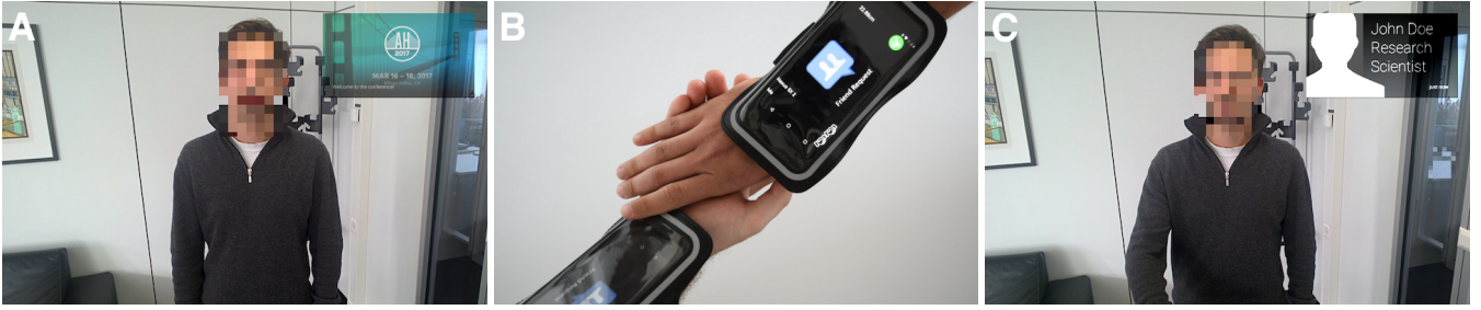
Figure 3: HandshakAR prototype. (A) The system is inactive. (B) The devices are in close proximity to each other and, at the same time, a handshake greeting gesture was recognized. The devices exchange contact information, in this case a Facebook friend request. (C) The contact information appears on the user’s HMD (the Google Glass in our prototype).
