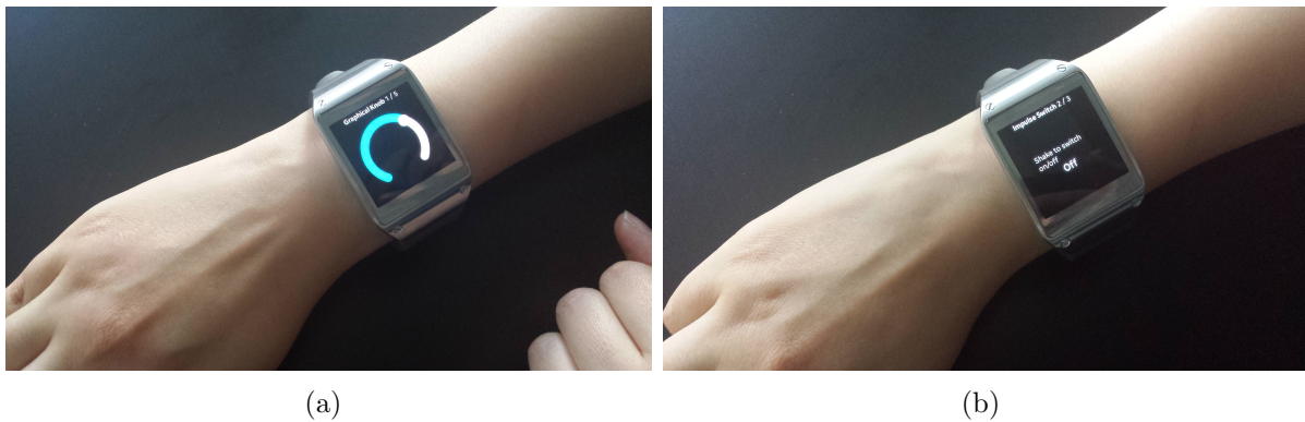
Figure 4.17: Interfaces for controlling a stereo set on a smartwatch: (a) A graphical interface to control the volume. (b) An interface that switches the stereo set on/off upon shaking the smartwatch.
