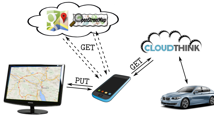
Figure 8.9: By publishing semantic metadata that describes its interfaces, functionality of CloudThink API (i.e., access to sensor values and actuators of connected vehicles) can be flexibly integrated with other local and remote Web services. In this example, a user instructs an interface device (in this case, a smartphone) to display the location of his car on a map that is shown on a nearby computer screen and a reasoner deduces the necessary HTTP requests.
