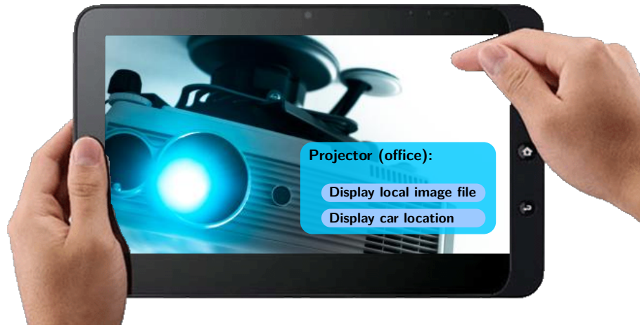
Figure 7.12: Using image recognition software and automatic deduction of user goals from RESTdesc descriptions (mock-up): a projector acts as a proxy for service mashups that it can form part of. In this case, the projector provides the service to either display an image that is stored on the tablet device, or to display the location of the user’s car on a map.
