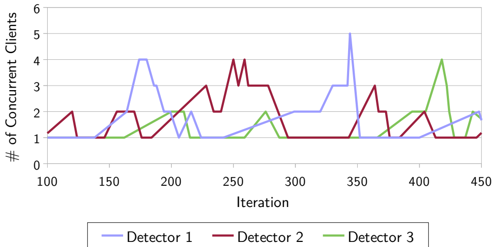
Figure 7.6: Illustration of the dynamic optimization capabilities of our marketplace implementation: 15 clients interact with three arrhythmia detection services. Of these 15 clients, three always select the same detector, seven request the cheapest detector, and five request the service with the lowest latency.
