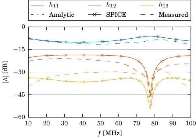
Fig. 4: Channel gains for a co-channel ( $h_{11}$ ), cross-channel of adjacent phases ( $h_{12}$ ) and of opposing phases ( $h_{13}$ ) of a branchless connection with matched terminations ( $100 \Omega$ ).
