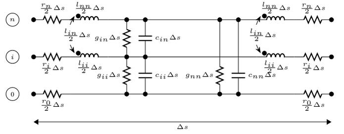
Fig. 3:  $T$ -model approximation of a transmission line segment of length  $\Delta s$ .
