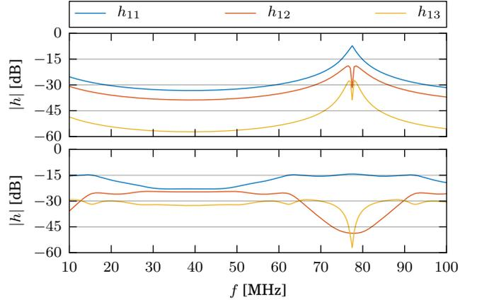
Fig. 5: SPICE-simulated CTF. Top: Branchless connection with low impedance ( $1 \Omega$ ) load. Bottom: Network with 3 branches and matched load.
