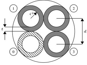
Fig. 2: Cross-sectional dimensions of cable bundle with 3 phases (grey insulation,  $i \in \{1, 2, 3\}$ ) and common return (striped insulation,  $i = 0$ ), conductor radius  $r_c$ , insulation thickness  $t$  and conductor distance  $d = 2(r_c + t)$ .
