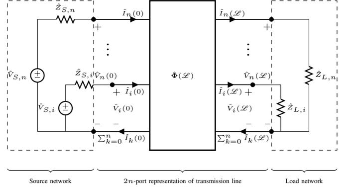
Fig. 1: Channel model for a MIMO PLC channel with  $n + 1$  conductors. The channel is modeled by a  $2n$ -port representation of the transmission line. Transmitter and receiver are modeled by source and load networks.
