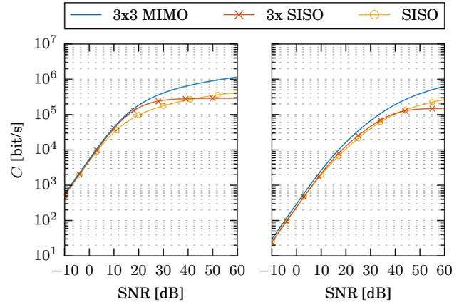
Fig. 6: Channel capacity for a direct connection between two nodes with matched line terminations (left) and low impedance ( $1 \Omega$ ) terminations (right).
