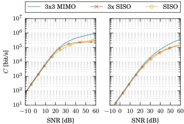
Fig. 7: Channel capacity for a connection with 3 branches and matched line terminations (left) and low impedance ( $1\ \Omega$ ) terminations (right).
