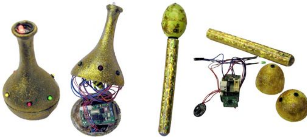
Figure 5.25: BTnode with RFID reader and sensor board embedded into a toy bottle (left) and a toy wand (right).
