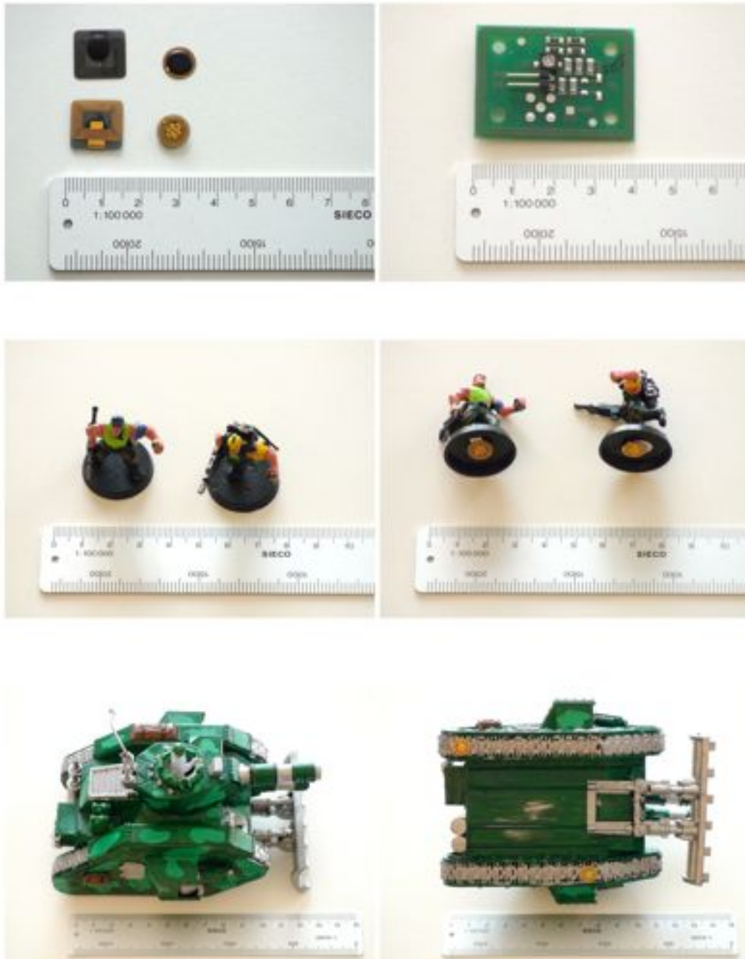
Figure 4.10: The RFID transponders used (top left) and the (small) RFID antenna we used (top right). In the middle there are two tagged game figures and at the bottom a large vehicle with two transponders.
