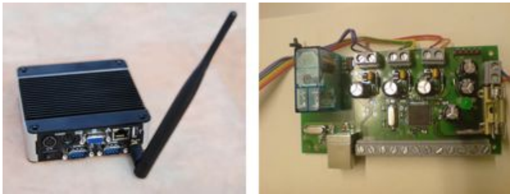
Figure 5.17: The NorhTec MicroClient Sr computer with a very small form factor (115x115x35 mm) (left) and the effect board (right).
