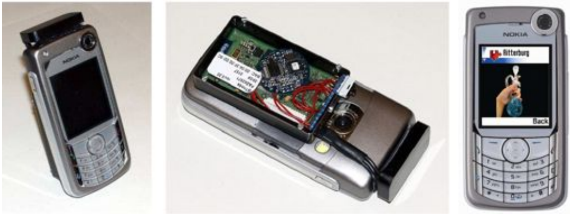
Figure 5.24: Mobile phone with RFID-reader and external antenna, front (left) and back view (center). The right picture shows its “embodiment” of a magic potion bottle.
