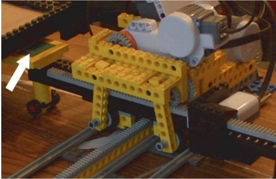
Figure 4.15: The robot moves the carriage with the antenna (indicated by the white arrow) using an orthogonal track system.
