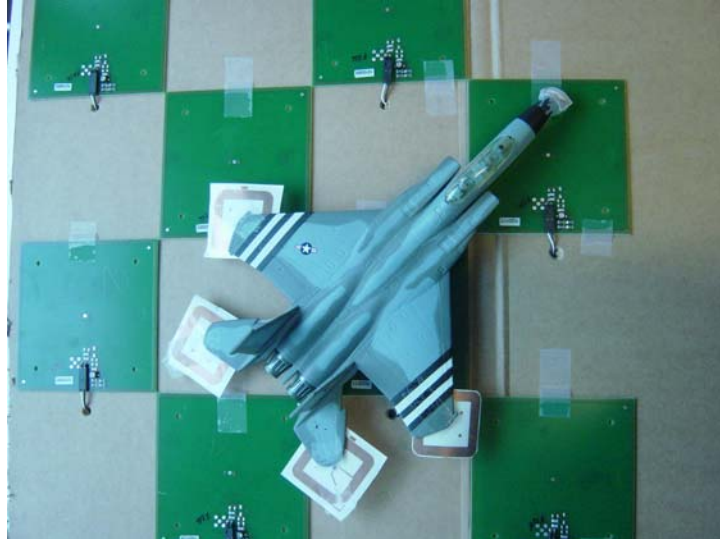
Fig. 8. Preliminary test with a multi-tagged object (using 4x4 centimetres RFID tags) and an antenna grid with 8 FEIG ID ISC.ANT 100/100.
