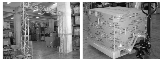
(a) Portal Reader [12] (b) Pallet with RFID Tagged Cases [12]
