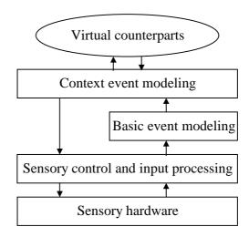
**Figure 6:** Layerd event-based architecture. After processing sensor input from the hardware, basic events are created and passed to the context event level, where events are held back, aggregated or released depending on context information.
