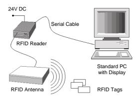
**Figure 7**: Schematic view of the RFID Chef hardware. The RFID reader antenna detects tagged artifacts in its vicinity and transmits raw sensory information through a reader module to the PC via serial cable.
