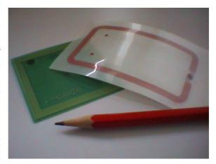
**Figure 8:** The two different form factors of I-Code RFID labels that are used in our RFID Chef testbed environment.
