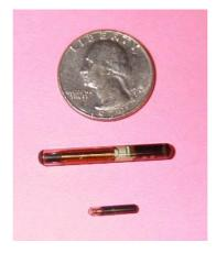
Figure 3: Typical form factors for RFID tags. The particular tags shown come in a glass casing in order to allow attaching them to metallic objects or to insert them below the skin of animals. (Image Source: Portolano Project [13])
