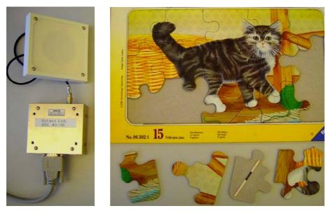
**Figure 4:** Hitachi  $\mu$ -chip RFID equipment used for building the Smart Jigsaw Puzzle Assistant prototype. In the left photo, one can see the RFID antenna and below the corresponding  $\mu$ -chip reader device by Hitachi. In the right photo, there is the physical puzzle game with four of its  $\mu$ -chip-tagged pieces shown underneath
