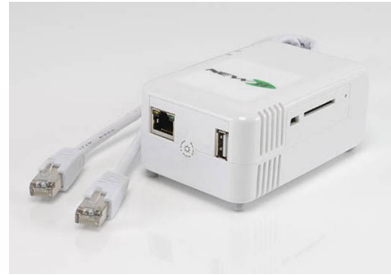
Figure 4.12: SheevaPlug mini computer to collect readings from the smart power outlets. [230]
