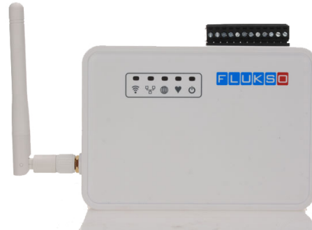
Figure 4.8: Fluksometer we used to query the data from the smart meter. [206]
