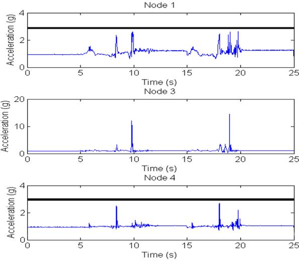
**Figure 8: Accelerations of Node 1 (chest), Node 3 (wrist), and Node 4 (thigh) for a slow fall caused by dizziness.**
