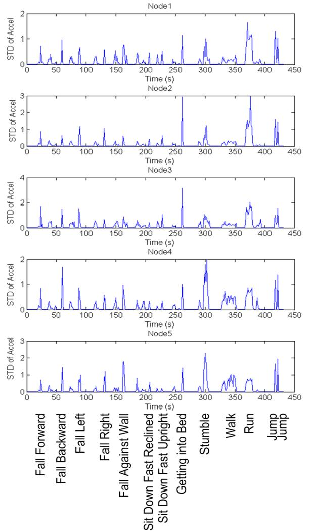
Figure 4: The standard deviation of the linear accelerations at the chest (Node 1), waist (Node 2), wrist (Node 3), thigh (Node 4), and ankle (Node 5) for various activities.
