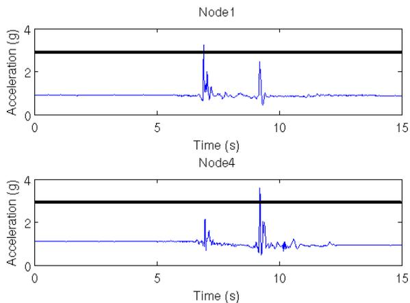
**Figure 10: Accelerations of Node 1 (chest) and Node 4 (thigh) for falling against wall**
