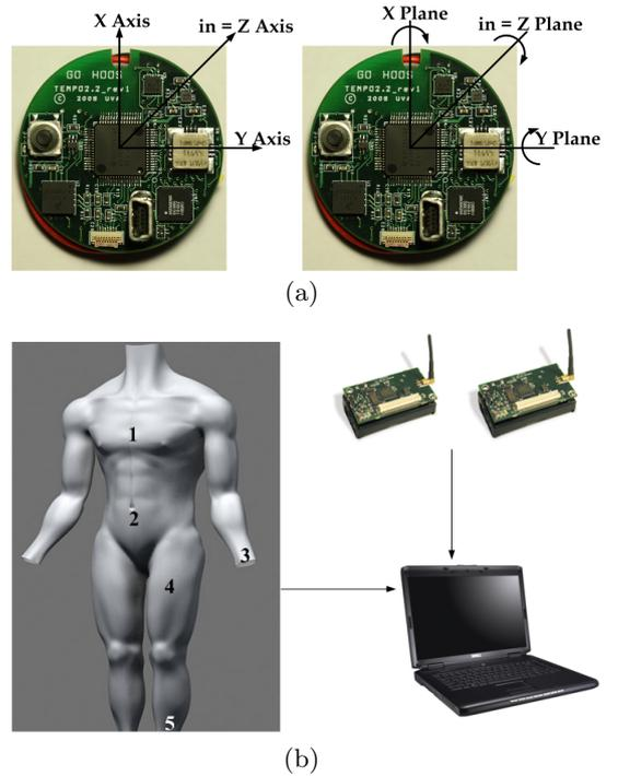
**Figure 1: (a) The TEMPO 3.1 sensor node; (b) The data acquisition system setup.**
