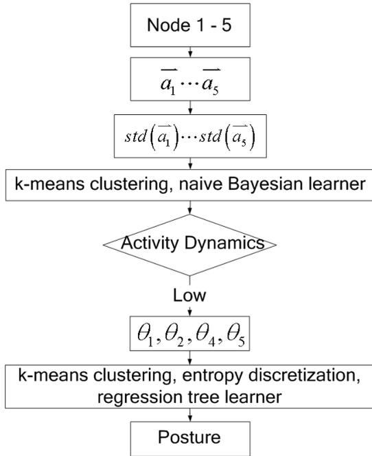
Figure 3: The process of posture recognition.
