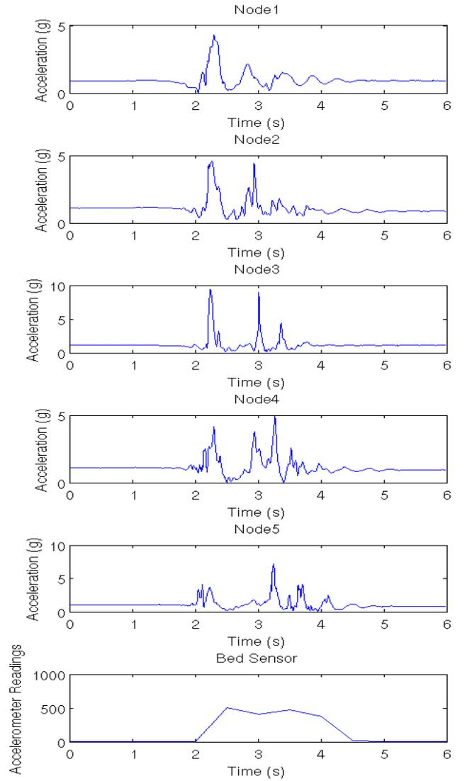
**Figure 9: Accelerations of Node 1 (chest), Node 2 (waist), Node 3 (wrist), Node 4 (thigh), Node 5 (ankle), and bed sensor for lying onto bed quickly.**
