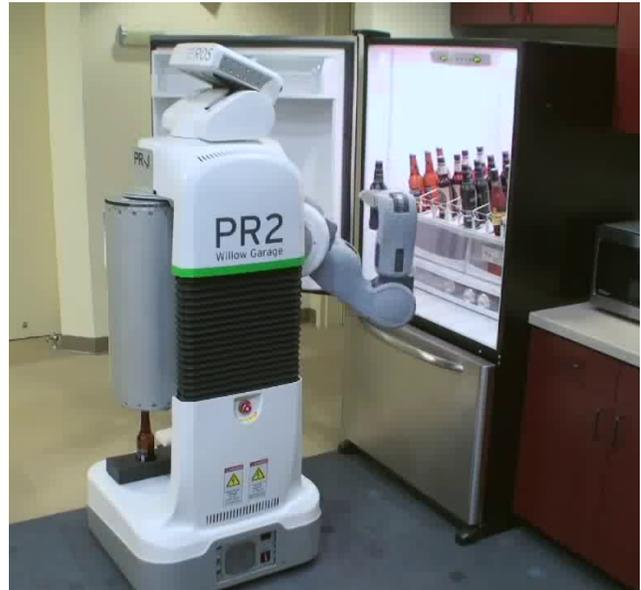
Figure 2: Willow Garage PR2, Robot for Research and Innovation [15].
