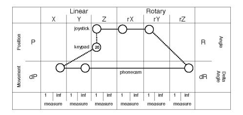
Fig. 3. Design space classification of our mobile phone prototype.
