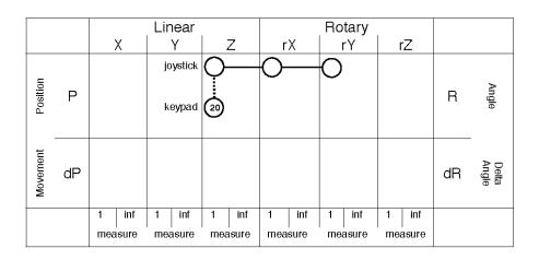
Fig. 2. Naive classification of mobile phone as an input device following the taxonomy presented in [15].
