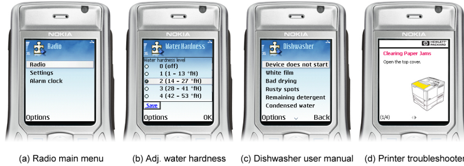
Fig. 1. AID prototype implementation. The screenshots show examples of the AID user interface for each of the four appliances used in the study. Appliance functions could either be selected by traversing the main menu (a) or by having the AID automatically (i.e., simulated, see Section 2.4) detect the appliance’s state (d).
