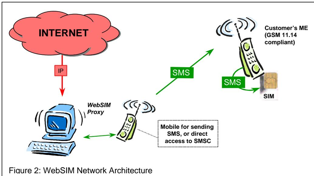
The connection between the Internet and the WebSIM is handled by a proxy host that tunnels HTTP-requests over SMS to the Web server applet in the SIM. Figure 2 shows the overall architecture: A HTTP-request arriving from the Internet for a particular WebSIM (determined by its phone number) is packed into a SM to the SIM, where the request is unpacked and processed. The response is sent back as a SM to the proxy, where a normal HTTP-response is send back to the originator in the Internet.
