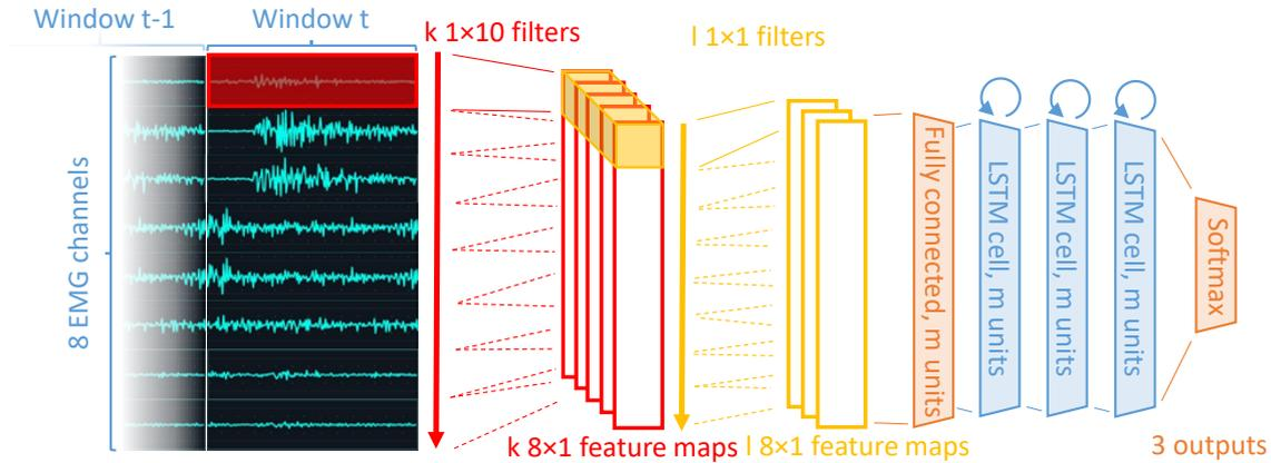
Figure 2.5: Our architecture for finger classification consisting of two convolutional layers with  $k$  and  $l$  filters, one fully-connected layer with  $m$  units, three stacked LSTM cells with  $m$  units each, and finally a softmax layer. The LSTM cells take five consecutive windows into account.
