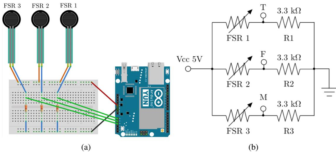
Figure 2.4: A diagram and the schematics of the hardware set-up for measuring the force values of finger presses showing the connections between the force-sensitive resistors and the Arduino.
