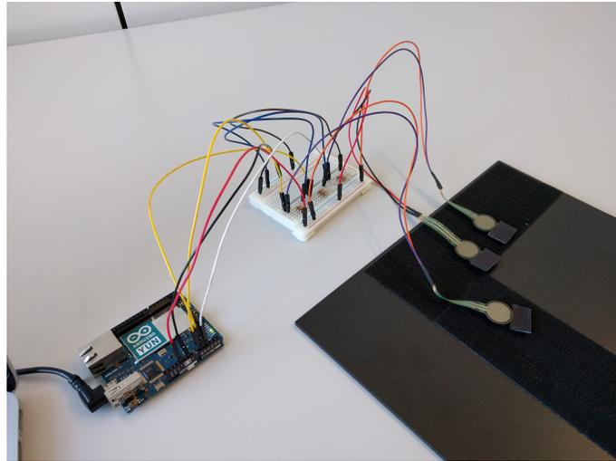
Figure 2.3: Our hardware set-up for collecting force ground truth consisting of a force-sensitive resistor for each of the three fingers (thumb, forefinger, and middle finger) and an Arduino.
