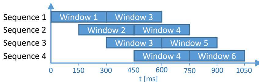
Figure 3.4: An illustration of how we segment the sequences (two consecutive windows) over time.
