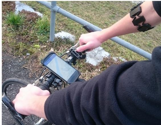
Figure 1.10: A user controlling the zoom setting of a map application with *TouchSense* without having to let go of the handlebars.
