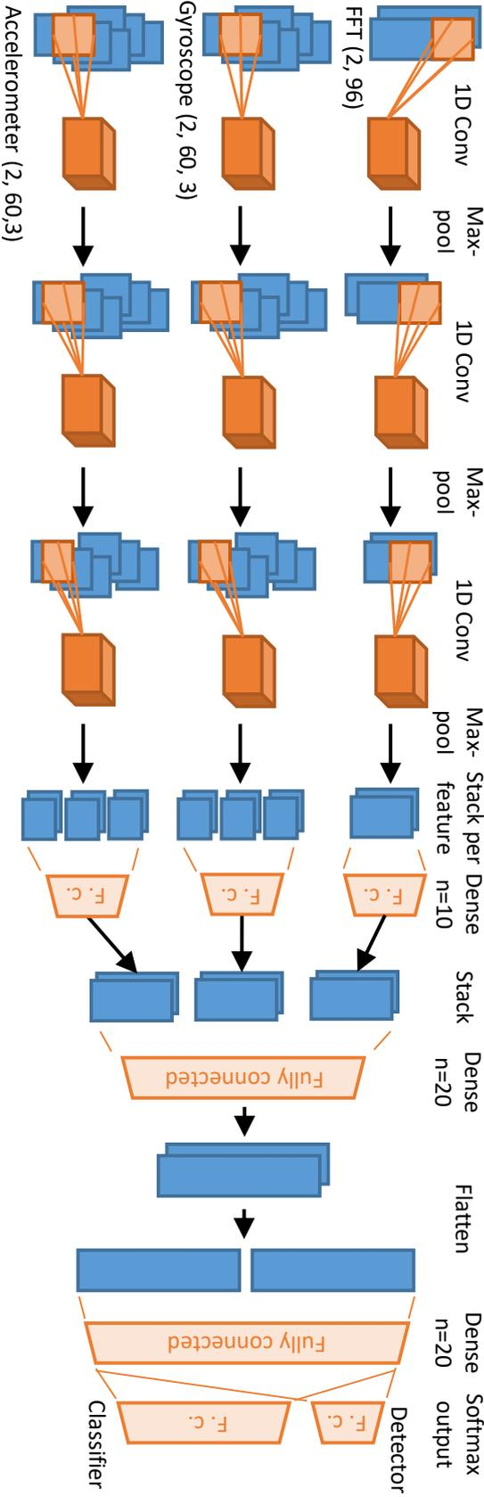
Figure 3.6: The neural network we designed for gesture recognition. The input are sequences containing two windows of audio spectra, and time-domain gyroscope and accelerometer data. The network consists of a convolutional part for extracting features from each input type separately, followed by fully connected layers which combine these features (F.c. stands for fully connected). It is responsible for both gesture detection and classification by providing two outputs.
