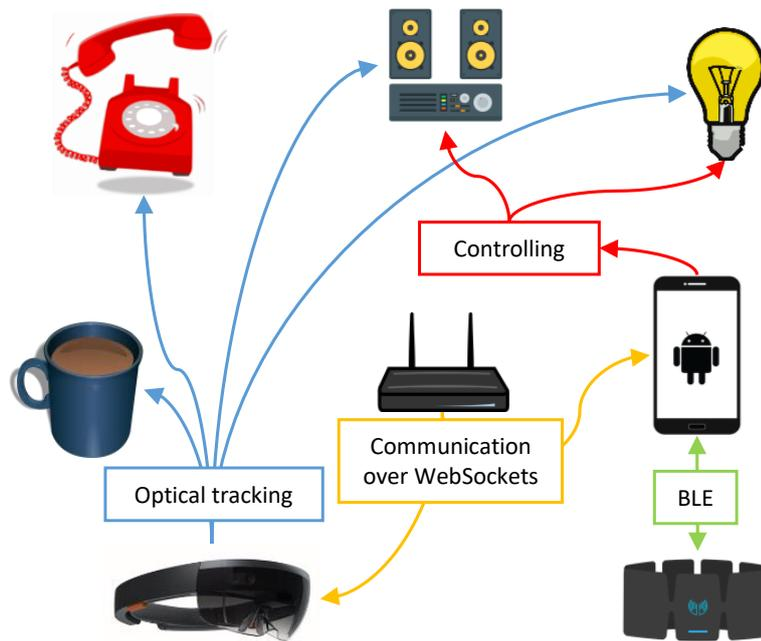
Figure 4.7: The HoloLens tracks the appliances and the mug (in Scenario 3). It communicates to the appliances and the Android smartphone via a Wi-Fi network. The Myo is connected to the smartphone via BLE.
