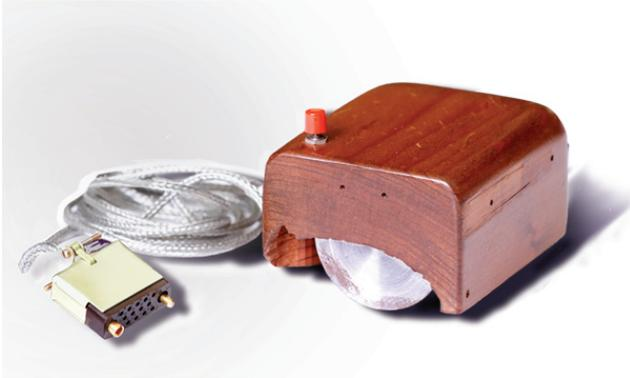
(a) A prototype of a computer mouse built by William English according to a design by Douglas Engelbart. Taken from [249].
