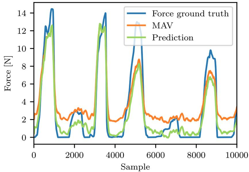
Figure 2.10: An example of the ground truth force values, the MAV, and the predictions of a linear regression model for 10,000 samples.
