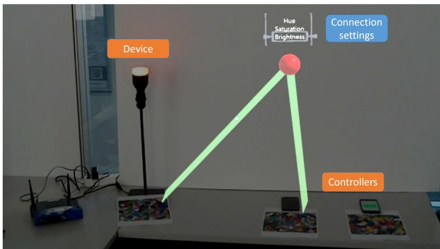
Figure 4.2: We present a second prototype for fast and simple configuration of device connections, such as between a common controller and a light, using simple gestures. The connections are visualized in augmented reality making it easy for the user to understand existing connections and to configure them. For simplicity, we use Android smartphones running an app as controllers.
