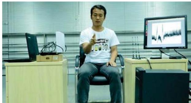
Figure 1.6: The *WiFinger* system recognizes gestures by measuring the distortion in the electromagnetic field between an emitting and a receiving Wi-Fi antenna. Taken from [113].
