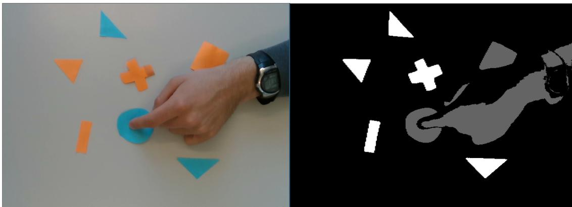
Figure 5.7: The binary shape masks with the detected hand region.
