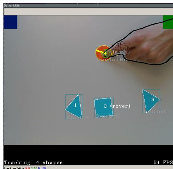
Figure 1.14: *Tailored Controls* recognizes the shapes the users produced and hand interactions upon them. These interactions can be forwarded to any application.
