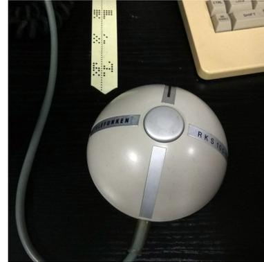
(b) A computer mouse developed by the German company AEG Telefunken. Taken from [245].
