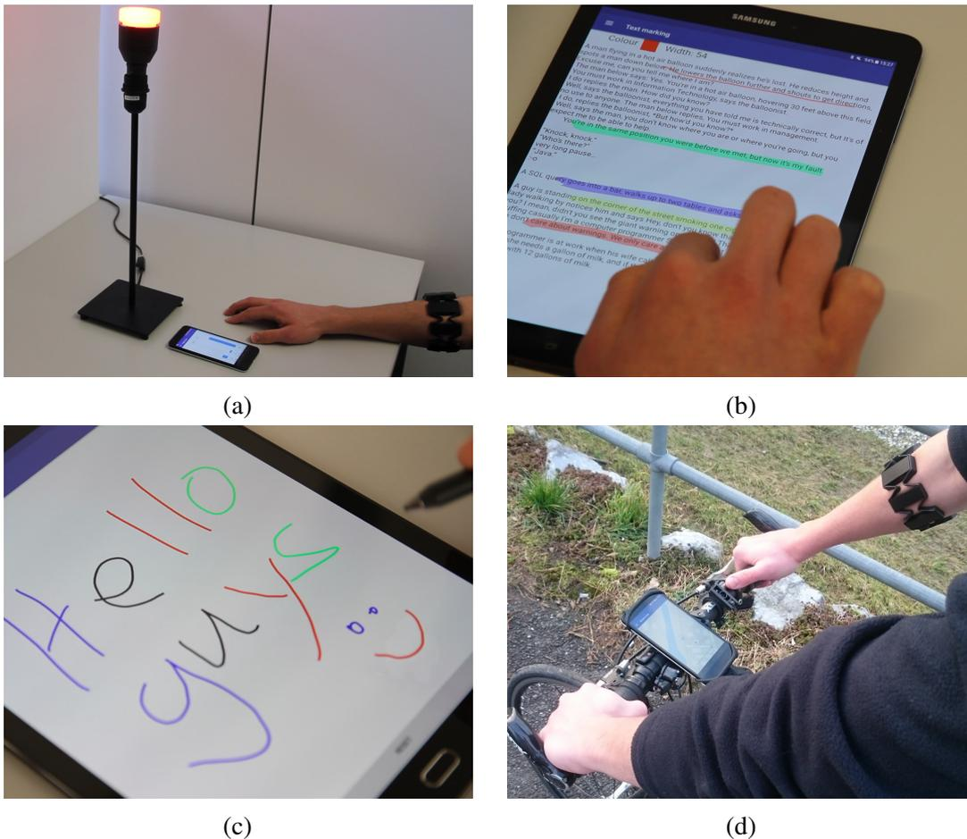
Figure 2.1: We propose a method that allows determining the finger and the force applied in touches. We present several applications using this method to enrich the interaction with devices.
