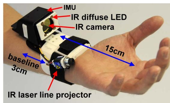
Figure 1.5: The *Digits* system incorporates a camera mounted on the user's wrist and hence can recognize gestures in any pose of arm and hand. Taken from [113].
