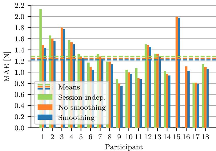
Figure 2.11: The mean absolute errors (MAE) when cross-validating linear regression models trained on the MAV and force ground truth from individual, and from multiple sessions.
