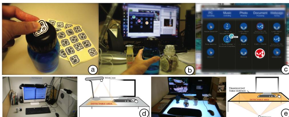
Figure 1.8: The iCon system allows a user to employ everyday objects as tangible user interfaces by attaching markers to the objects through which they are then tracked. Taken from [218].
