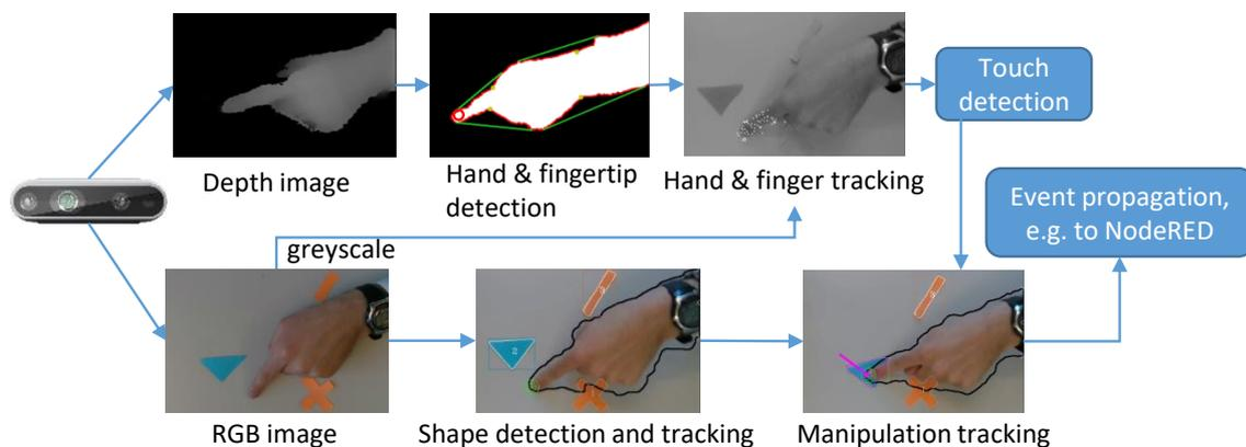
Figure 5.5: Our processing pipeline mainly consisting of finger and shape tracking based on the images from the depth camera.
