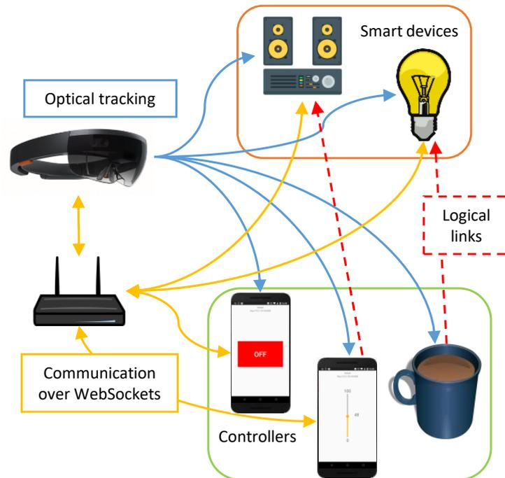
Figure 4.16: The HoloLens tracks the smart devices and the controllers. It communicates to the devices and the controllers via a Wi-Fi network, which is established by a router. The logical control link between a controller and a device is established once the user selects these and their potential connection is valid.
