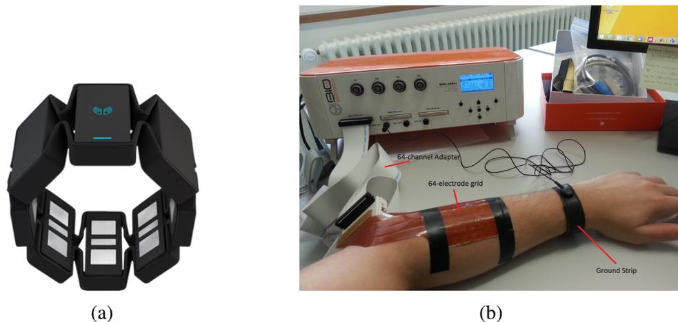
Figure 2.2: The wireless Thalmic Labs Myo (picture taken from [238]) compared to a traditional EMG recording set-up.
