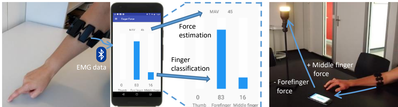
Figure 1: We propose a method which can turn any surface into a force-sensitive input modality by augmenting the user with an inexpensive and wireless EMG armband and a smartphone for running finger classification and touch force estimation. This enables new ways of interacting with appliances, such as a lamp for example.
