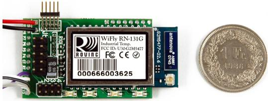
**Figure 2: The Roving RN-134 evaluation board, which includes an RN-131.**
