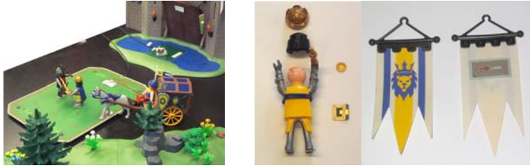
Fig. 5. Antennas embedded in the playset (left) and RFID transponders to tag toy pieces (right)
