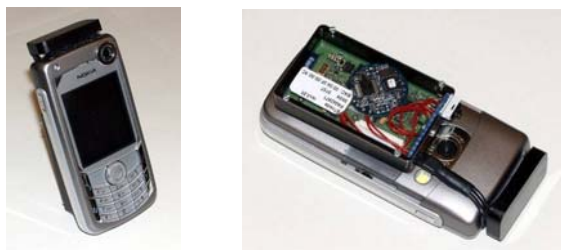
Fig. 5. Nokia 6830 with BTnode-RFID-reader and external antenna (front and back view)
