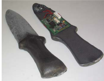
Fig. 7. BTnode with mobile RFID reader embedded into a toy sword
