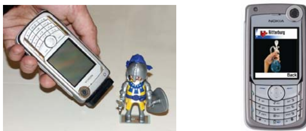
Fig. 6. Point-me, touch-me interaction between mobile phone and figure (left) and a mobile phone that takes on the role of a magic potion (right)
