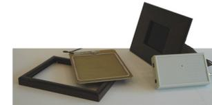
The **FEIG PR100 RFID reader** is unobtrusively embedded in the picture frame connected to a **custom built antenna**, which is molded into the stage allowing for close proximity to the exhibited collectibles.
