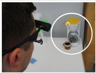
**Figure 2:** ubiGaze: an augmented reality system that allows embedding virtual messages into any object through gaze gestures [1]. Gaze gestures are captured using the Pupil wearable eye tracker.
