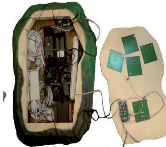
Figure 3 AKC internal RFID technology, antennae (right hand side), multiplexers and surround sound inside main housing (see online version for colours)
