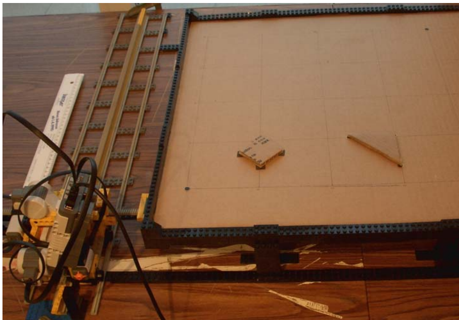
Fig. 6. The test environment with the robot, the carriage, and the tracks as well as the cardboard surface with two test objects. The two objects have RFID transponders attached to each of their corners.
