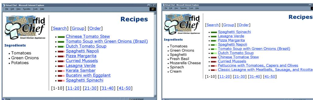
**Figure 4:** Sample screenshot of the *RFID Chef* prototype implementation. On the left side, three ingredients have been placed on the counter: tomatoes, green onions and potatoes. The system suggests a Chinese tomato stew. After the potatoes have been removed and five additional ingredients have been put on the counter, the recipe list dynamically adapted to suggest Spaghetti Spinachi instead.
