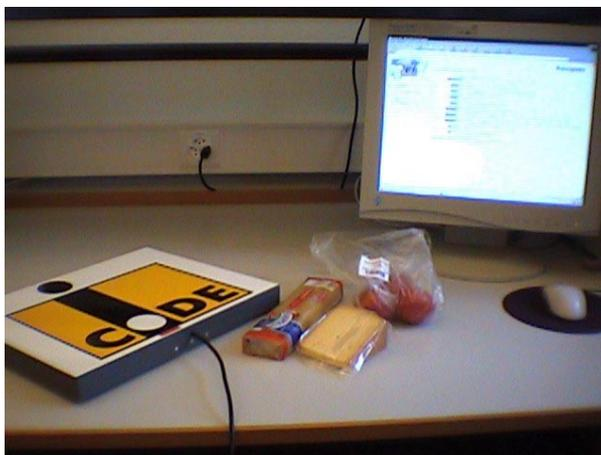
**Figure 5:** Experimental setup of RFID Chef in our lab. A standard office desk functions as our kitchen counter, an 18” LCD monitor acts as our display. Several individual ingredients have been placed on the table, where an RFID antenna (here shown in its casing, next to the ingredients) detects them and reports their presence to a PC that controls the display. Note that the antenna is usually mounted underneath the table.
