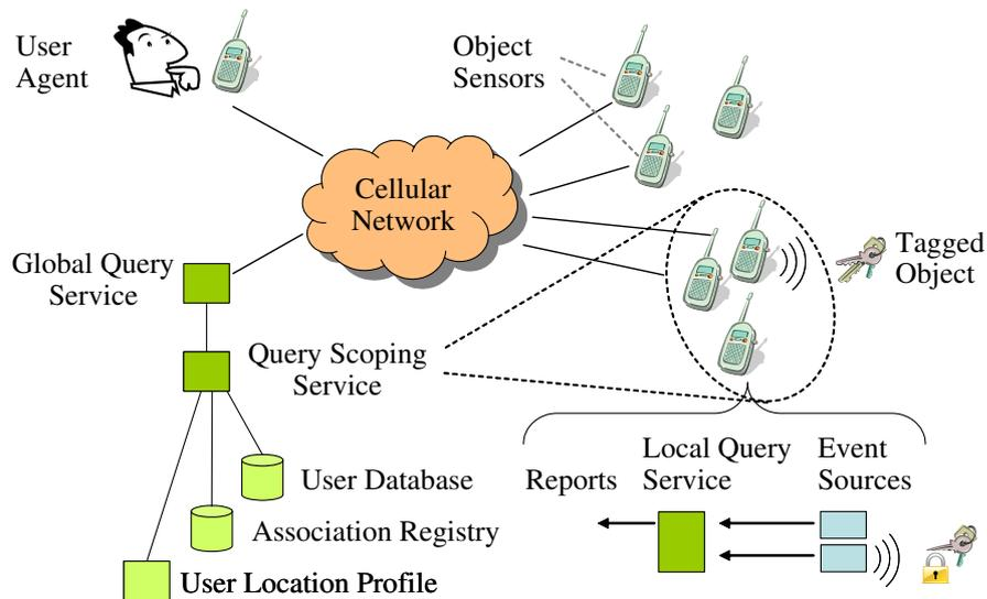
Figure 4.2: System architecture
