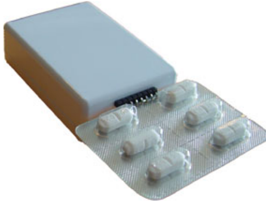
Fig. 1. Smart Blister Pack: A conventional blister pack is equipped with sensors to detect the removal of pills. The blister pack is attached to a communication module, which observes the “pill” sensors and transfers the compliance data to the patient’s mobile phone.
