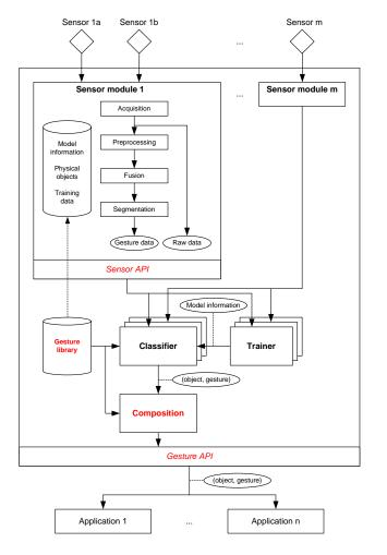
Framework for orientation sensor-based gesture recognition
